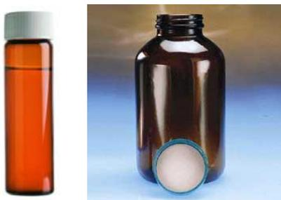
Glass bottles must be used. The type of cap required will depend upon the analyte and method the lab is using. Talk to the lab to be sure.
